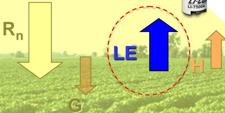
$$LE = L\rho_a \overline{w'q'} = \frac{J}{g H_2O} \times \frac{g \text{ air}}{m^3} \times \frac{m}{s} \times \frac{g H_2O}{g \text{ air}} = \frac{J}{m^2 s} = \frac{W}{m^2}$$
